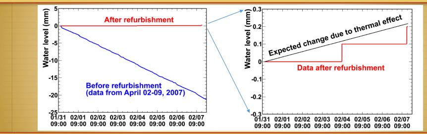
Currently we do not observe any water leakage from the SK tank within the accuracy of our measurement, which is less than 0.017 tons per day.
