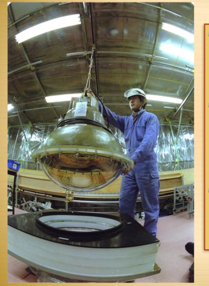
The photo-multiplier-tubes (PMTs) support structure divides the tank into two distinct, optically isolated volumes, the inner detector (ID) and the outer detector (OD).
