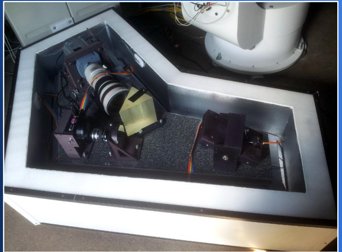
fiber-fed, echelle spectrograph, R \sim 40000
