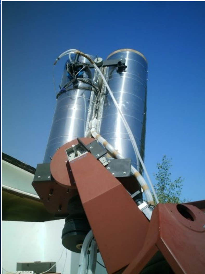
2 x 0.5m telescope with fiber fed echelle spectrograph
