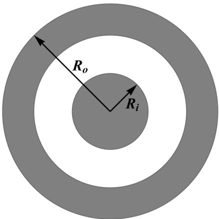
**Figure 1:** Weakly doped bilayer graphene ring characterized with inner  $R_i$  and outer radii  $R_o$  between metallic contacts.
