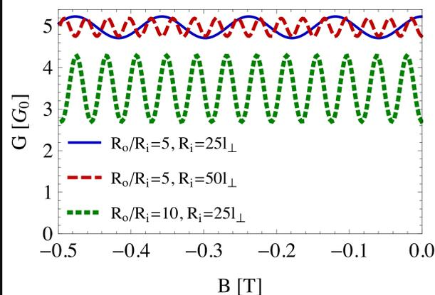
**Figure 2:** Oscillatory behavior of conductance at the Dirac point for three different setups. Note that the amplitudes as well as average conductance depend only on the ratio whereas the period depends on the size of the sample as well.
