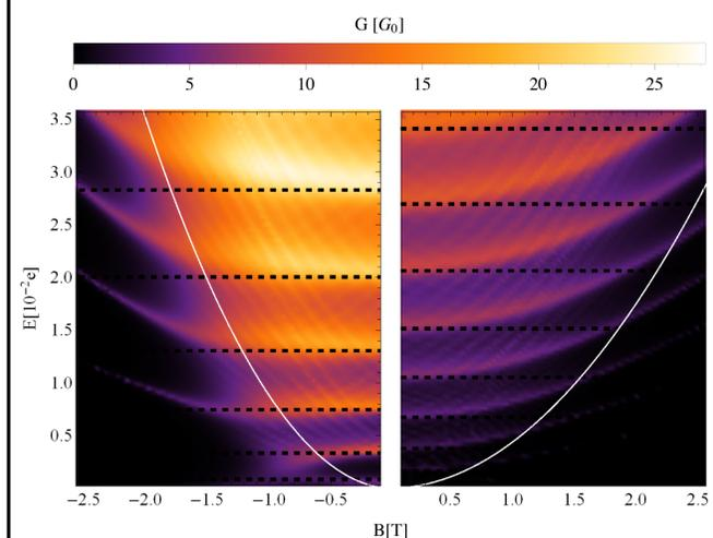
**Figure 4:** Comparison of conductance as a function of doping and magnetic field of bilayer graphene (left) and 2DEG (right) disks with the same inner and outer radii  $R_i = 25l_\perp$  and  $R_o = 100l_\perp$ . Dotted lines indicate quantum-well-like resonances, white lines depict the ballistic regime limit marked by the cyclotron radii.
