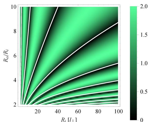
**Figure 3:** Relation between oscillation amplitudes in bilayer and monolayer graphene. (a) White lines follow Eq. (6) for vanishing oscillations in bilayer graphene. (b) Ratio between oscillations in bilayer and monolayer graphene for two selected inner radii.
